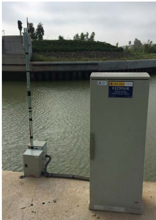
Figure 4. A sensor for tide height installed in the “Gate of the Sea” lock at the entrance of the Port facilities in the city of Seville. This sensor is wirelessly linked to the integration platform.
