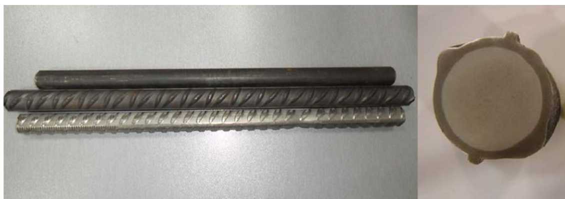
FIGURE 1. Reinforcing bars used in this study. (Left) Carbon round, carbon rebar and stainless steel rebar; (Right) Tempcore ® structure of the carbon steel.
