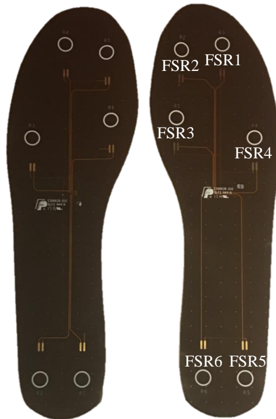
Figure 7: Fabricated insoles with FSR's location
