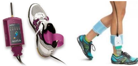
Figure 2: Novel's Pedar and Tekscan's F-Scan system
