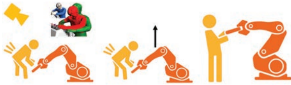
Fig. 1. Example application scenario of the WPC. The first 2 images show a non-optimal pose of the work piece forcing the human to adopt awkward posture when working on it. The last image shows a configuration leading to a natural work posture.
