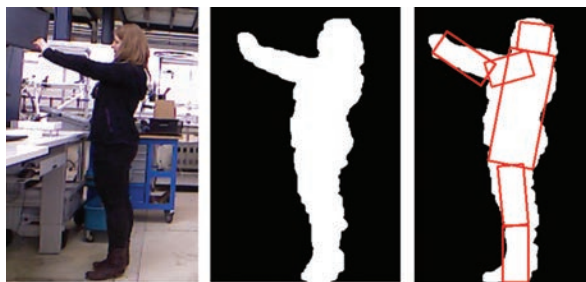
Fig. 3. Tracking work flow: Color image (left), segmentation mask of the subject (center), optimised human model (right).
