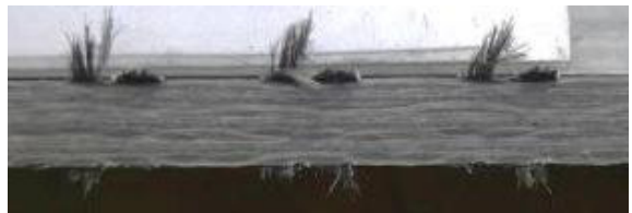
Fig. 5. Workpiece quality for end mills out of different cutting materials during peripheral milling of CFRP.
