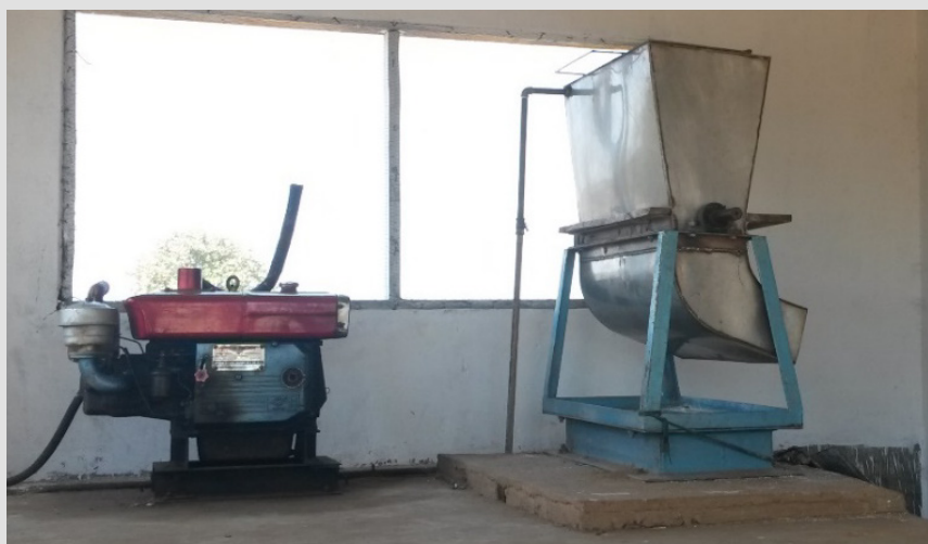
Cassava grater (right) and diesel generator (left) in a rural processing unit
