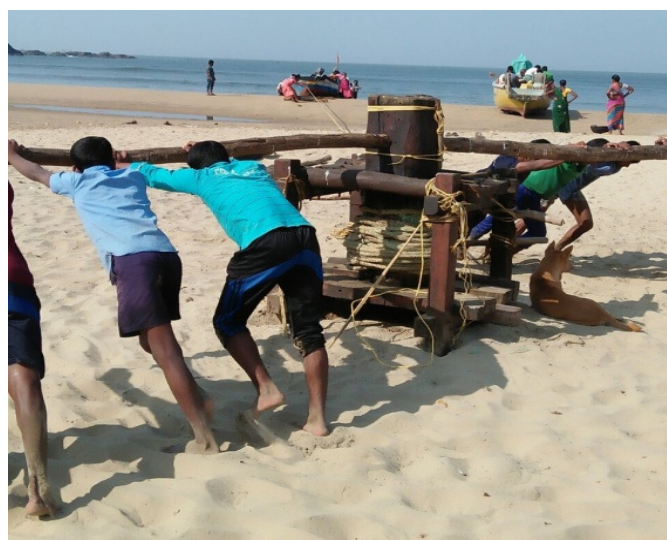
Figure-3: Fishermen rotating the pivot using the handle and hauling the boat onto the beach.
