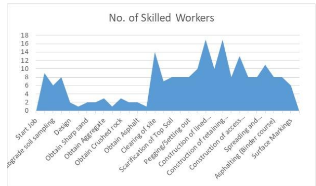
Fig. 2: Shows the number of skilled workers needed for each job.
