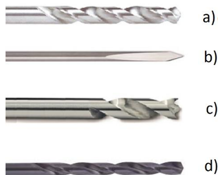
Figure 1: Drill geometries used: a) Twist; b) Dagger; c) Brad; d) HSS.
