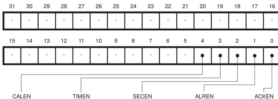
Figura A.12: Formato del registro RTC Interrupt Enable Register
