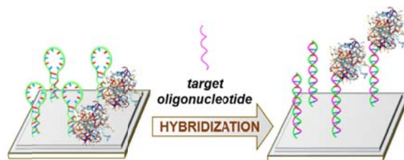
Figure 2 Scheme of the hybridization events for the streptavidin-free and the streptavidin-labeled MB probes being immobilized on the surface of a photonic structure.
