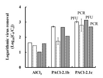
Figure 6. Comparison of removal ratios of PV (white) and CV (gray) after settling during the coagulation process at approximately pH 7. Source water, lake water; coagulant dosage, 2.70 mg-Al/L. Values were determined from one experiment or are the means of duplicate experiments; error bars indicate the data range.
