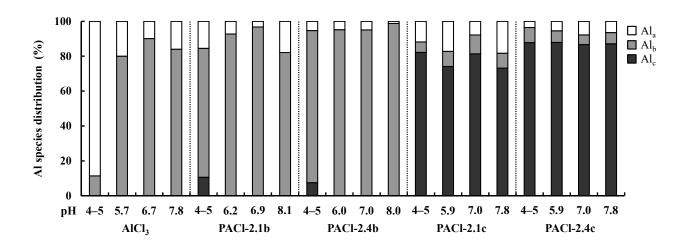
Figure 4. Effect of pH on the transformation of aluminum species after coagulant dosing, as evaluated by using the ferron method.
