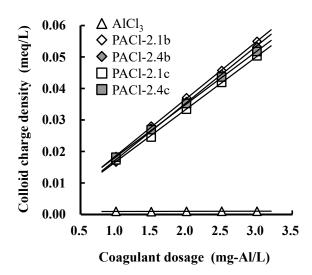
Figure 5. Positive colloid charges of the coagulants used in the present study, as evaluated by using the colloid titration method.
