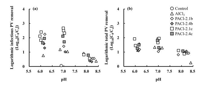
Figure 3. Effect of aluminum hydrolyte species in coagulants on (a) infectious PV removal as evaluated by using the PFU method and on (b) total PV removal as evaluated by using the PCR method after settling during the coagulation process. Source water, river water; coagulant dosage, 1.08 mg-Al/L.
