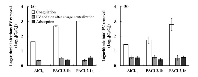
Figure 7. Effects of charge neutralization and adsorption on preformed aluminum floc particles on (a) infectious PV removal as evaluated by using the PFU method and on (b) total PV removal as evaluated by using the PCR method during the coagulation process at approximately pH 7. Source water, lake water; coagulant dosage, 2.70 mg-Al/L. Values were determined from one experiment or are the means of duplicate experiments; error bars indicate the data range.
