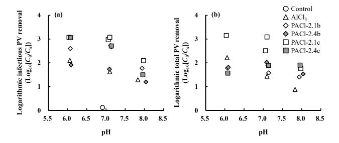
Figure 2. Effect of aluminum hydrolyte species in coagulants on (a) infectious PV removal as evaluated by using the PFU method and on (b) total PV removal as evaluated by using the PCR method after settling during the coagulation process. Source water, lake water; coagulant dosage, 2.70 mg-Al/L.
