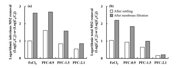
Figure 2. Effect of the basicity of polyferric chloride (PFC) on infectious MS2 removal as evaluated by using a plaque-forming unit method (a), and total MS2 removal as evaluated by using a real-time polymerase chain reaction method (b) after settling and after membrane filtration at pH 6. Coagulant dosage, 4.48 mg-Fe/L. The numbers after "PFC" represent the basicity of the coagulant.
