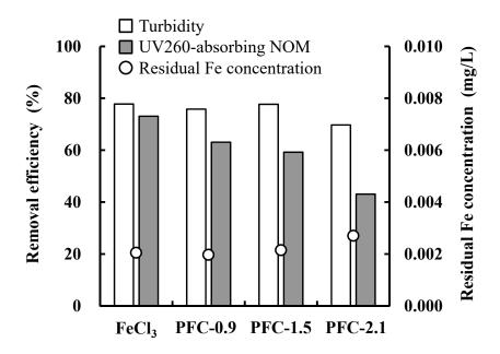
Figure 1. Effect of the basicity of polyferric chloride (PFC) on removal of turbidity and UV260-absorbing natural organic matter (NOM), and residual Fe concentration after settling, after coagulation at pH 6. Coagulant dosage, 4.48 mg-Fe/L. The numbers after "PFC" represent the basicity of the coagulant.
