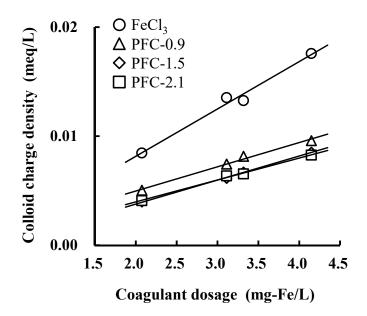
Figure 5. Positive colloid charge densities of the polyferric chloride (PFC) coagulants used in the present study as evaluated by means of a colloid titration method. The numbers after "PFC" represent the basicity of the coagulant.
