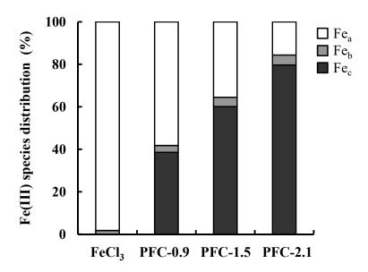
Figure 4. Distribution of iron(III) species in the polyferric chloride (PFC) coagulants used in the present study as evaluated by a ferron method. The numbers after "PFC" represent the basicity of the coagulant. Fe<sub>a</sub>, monomeric species; Fe<sub>b</sub>, polymeric species; Fe<sub>c</sub>, precipitated species.
