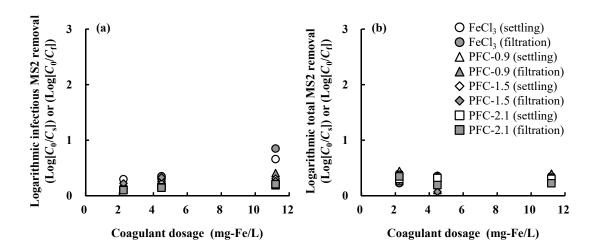
Figure 3. Effect of the basicity and dosage of polyferric chloride (PFC) on infectious MS2 removal as evaluated by using a plaque-forming unit method (a), and on total MS2 removal as evaluated by using a real-time polymerase chain reaction method (b) after settling and after membrane filtration at pH 8. The numbers after "PFC" represent the basicity of the coagulant.
