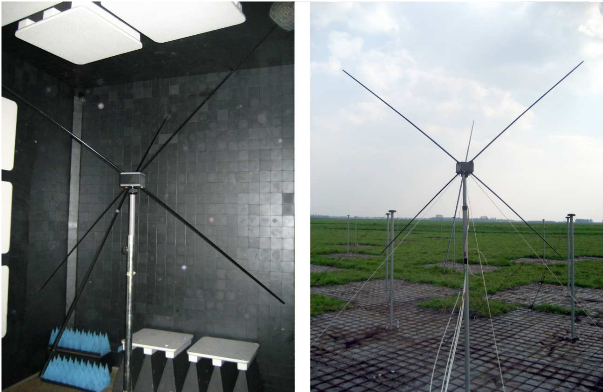
Figure 14: Tests with the prototype tripole antenna [13]. Left: Test setup in ASTRON chamber. Right: Setup in LOFAR station CS011 with 2 meters above the ground.
