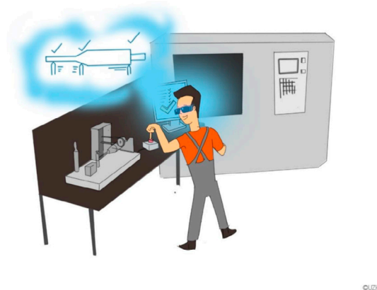
Figure 3. Using the measuring device in combination with AR glasses, a machine operator can immediately see the digitally augmented measurement results (FACTS4WORKERS 2015).
