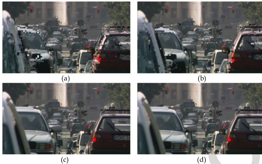
Fig. 13. Subjective video quality comparison of 1362nd frame (captured at sink device #4): (a) Pseudo-broadcast, (b) DirCast, (c) ACK-based multicast, and (d) proposed system.
