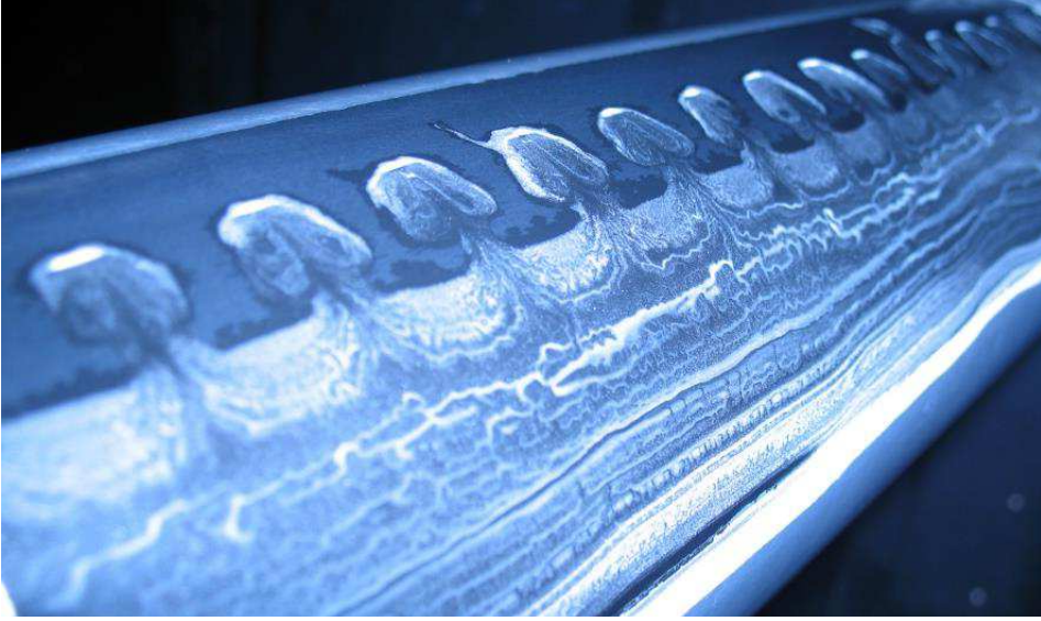
Figure 12: Surface oil flow pattern obtained by applying oil mixture to the rear side of the cylinder. The jet spacing and Reynolds number are identical to those used for figure 11.
