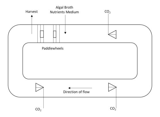
Fig. 1-2 Plan view of a raceway pond. Nutrient input is inserted after the paddlewheel and executes a cycle while being aerated with Carbon Dioxide. It is harvested before the paddlewheel to begin another cycle (adapted from Brennan and Owende, 2009).
