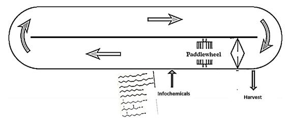
Fig. 1-7 Schematic representation of potential application of naturally occurring zooplankton infochemicals in open raceway ponds, per Industrial Ecology principles
