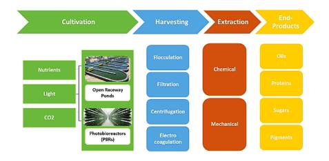
Fig.1-1 Diagram of production cycle and possible products obtainable from algal biomass
