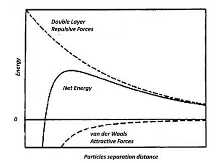
Figure 1-5 Schematic Representation of the DLVO theory
