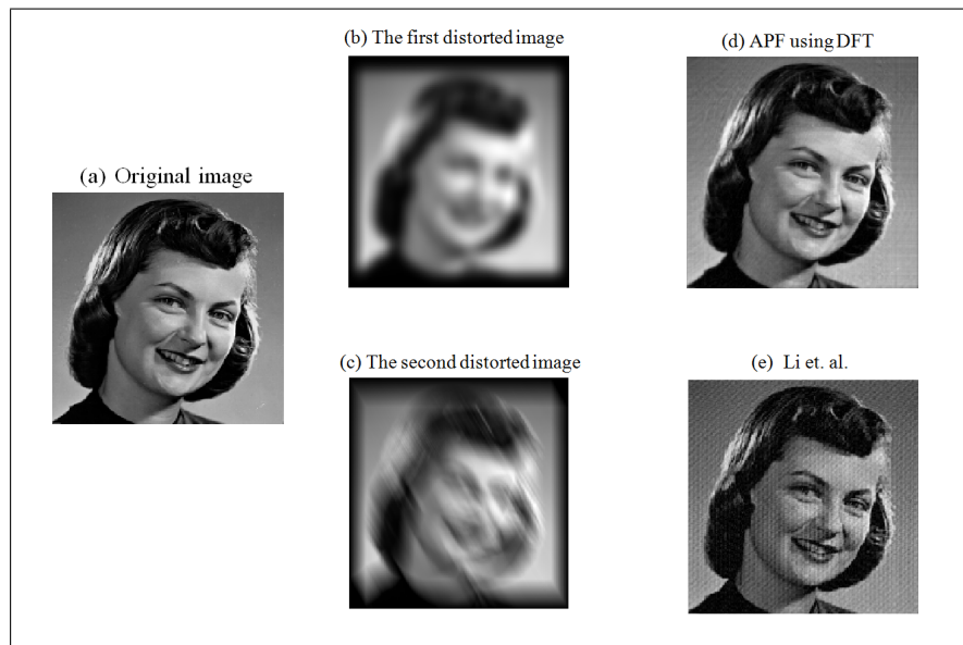
FIGURE 6.7: Blind Image Deconvolution of a noisy blurred image using (d) the developed method and (e) the method developed by Li et al. [1, 2], for Example 6.1.
