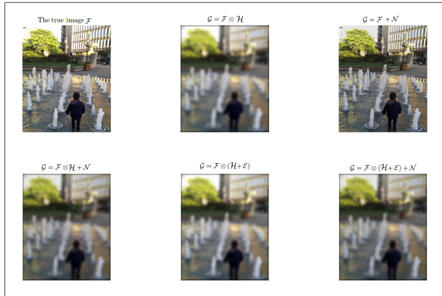
FIGURE 2.3: Five common cases of blurred images depending on the impact of artefacts on the image.
