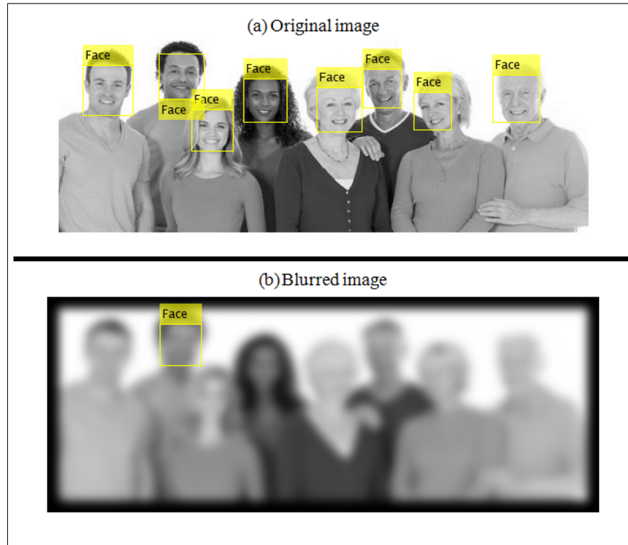
FIGURE 7.16: The face detector results using (a) the original image and (b) the blurred image.
