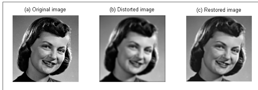
FIGURE 2.8: Image de-blurring using Wiener filter. (a) an clear image; (b) a blurred image; and (c) the restored image.
