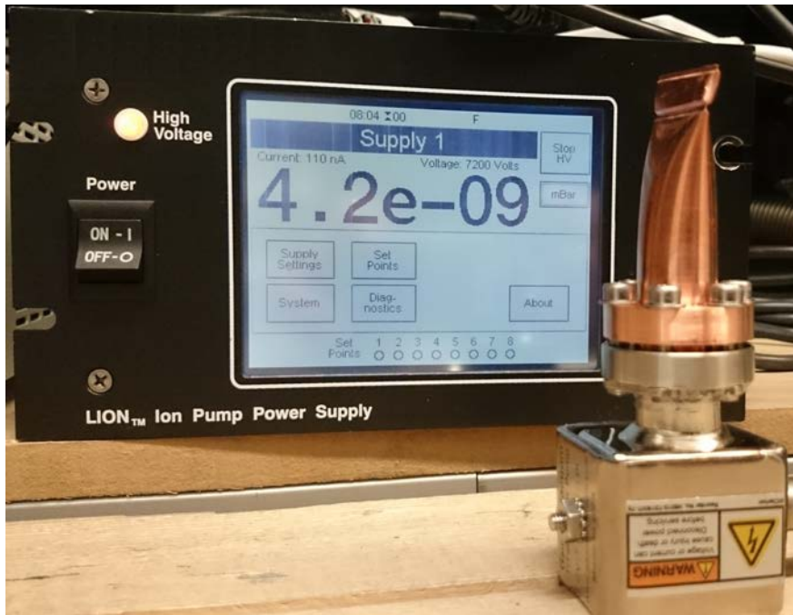
Figure 4.18: Ion pump with an attached compression valve. The ion pump controller is visible in the background, showing the pressure in units of mbar.
