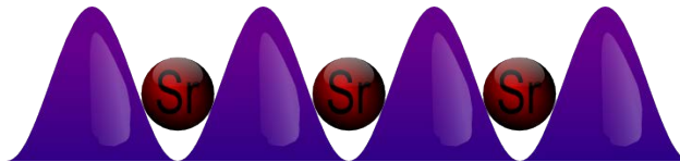
Figure 3.9: After two stages of cooling, atoms are confined in an optical lattice. An optical lattice is an optical potential that is created when counter-propagating beams of light create a standing wave.
