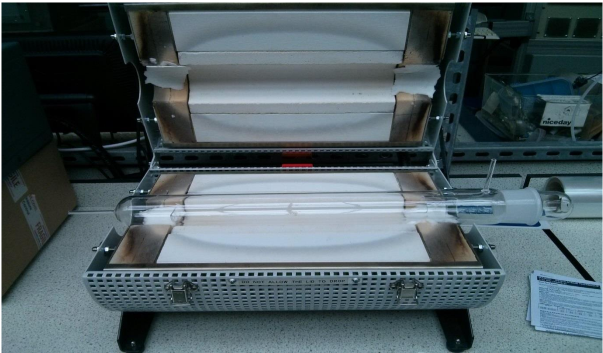
Figure 3-1 Quartz tube and furnace for anode sample testing. Fuel gas enters from the left hand side, passes over the samples which are resting across a alumina plate.
