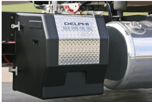
Figure 1-3 Example of SOFC APU unit from Delphi. [2] The unit provides electricity and heat inside of long-haul trucks.
