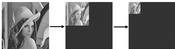
Fig. 2. A two-level HDWT four-band split of "Lena".
