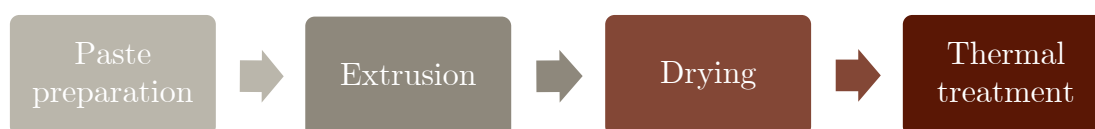
Figure 8 - Stages of the formulation process by extrusion.
