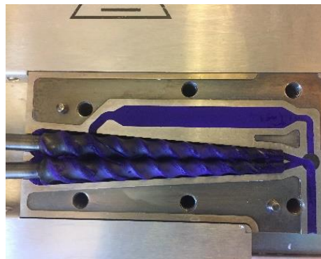
Figure 15 - Extruder compartment following 5 minute, closed-cycle extrusion.
