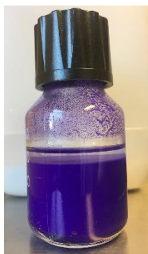
Figure 13 - Preliminary step: UTSA-16 soaking in propanol.
