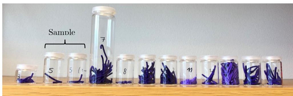
Figure 21 - UTSA-16 extrudates following extrusion and activation.
