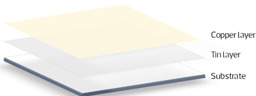
Figure 5.1 - Thin film metallic layer sputtering deposition example scheme.
