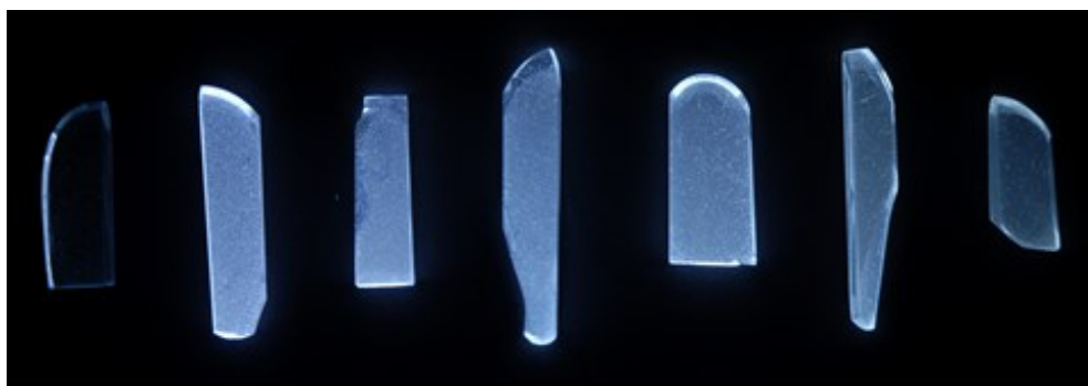
Figure 3.1 - Tin oxide doped samples under 5.16 eV excitation wavelength, from left to right: BG-0%Sn, T1-0.4%Sn, T2-0.7%Sn, T3-1.1%Sn, T4-1.4%Sn, T5-2.7%Sn, T6-3.4%Sn.
