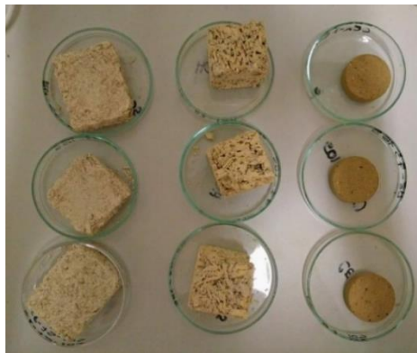
Figure 3.1- Example of samples used in sorption isotherm test - Earth plaster on the left, hemp concrete in the middle and compacted earth on the right.
