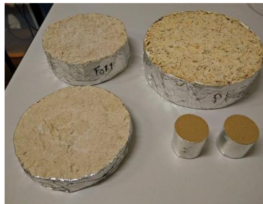
Figure 3.2- Example of samples used in MBV test - Earth plaster on the left (with two thicknesses: 2cm and 4cm), hemp concrete on the superior right corner and compacted earth on the inferior right corner.
