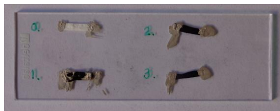
Figure 2.3 - Optical camera image of an example preparation with different functionalized CA membranes, (PANI/CA, PPy/CA and PEDOT/CA), which were cut and immobilized on microscope slides with silver conductive glue to measure electrical conductivity
