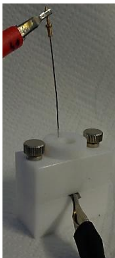
Figure 2.6 - Picture of the electrochemical Teflon-made cell used on the Cyclic Voltammetry studies.
