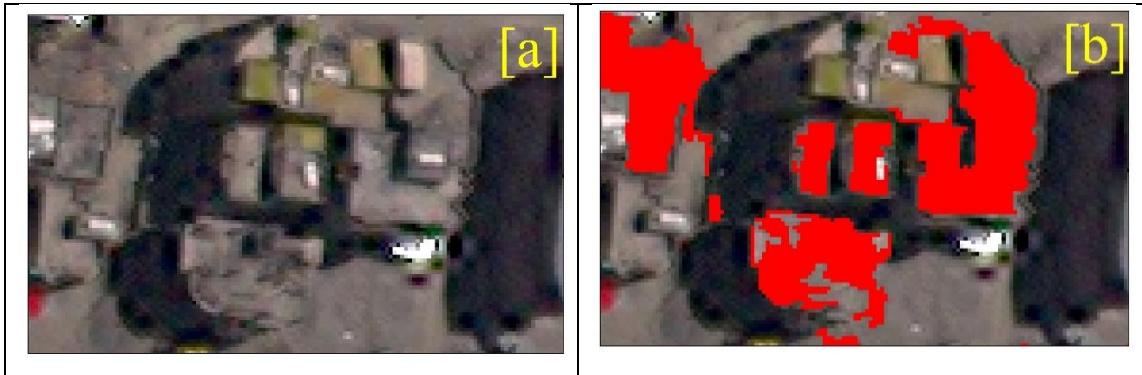
Figure 13. Example of misclassified class in subset 2. [a] under construction site in the study area [b] example of under construction building classified as slums due to the geometric similarity with slum buildings.
