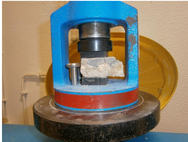
Figure 3 – General view of the applied compressive strength test
