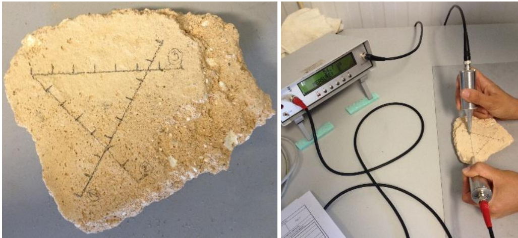
Figure 4 – Images showing a sample marked for the application of dynamic modulus of elasticity test (left), and the test being performed (right)
