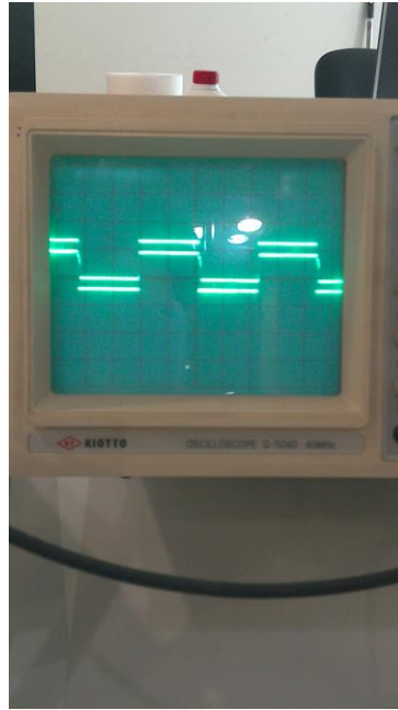
Figure 23 - Input and output signals on the oscilloscope, with an input wave of 200 Hz and the output wave saturated at 5 V.
