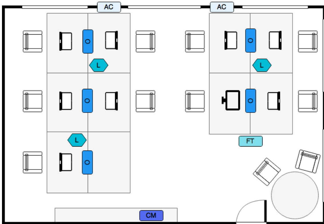
Figure 3.1: SmartLab simplified 2D model. Legend: AC - Air Conditioning, CM - Coffee Machine, FT - Fish Tank, L - Light Bulb, O - Outlet
