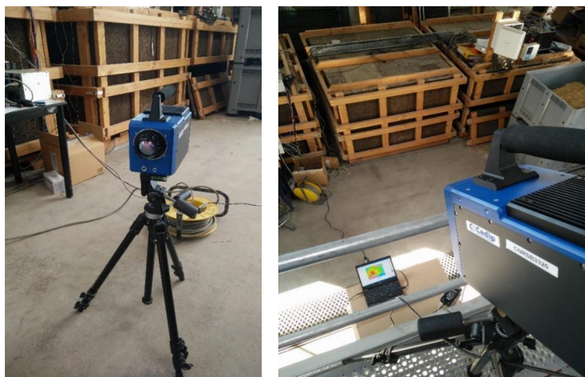
Figure 3.16 - Infrared camera analysing the chamber
