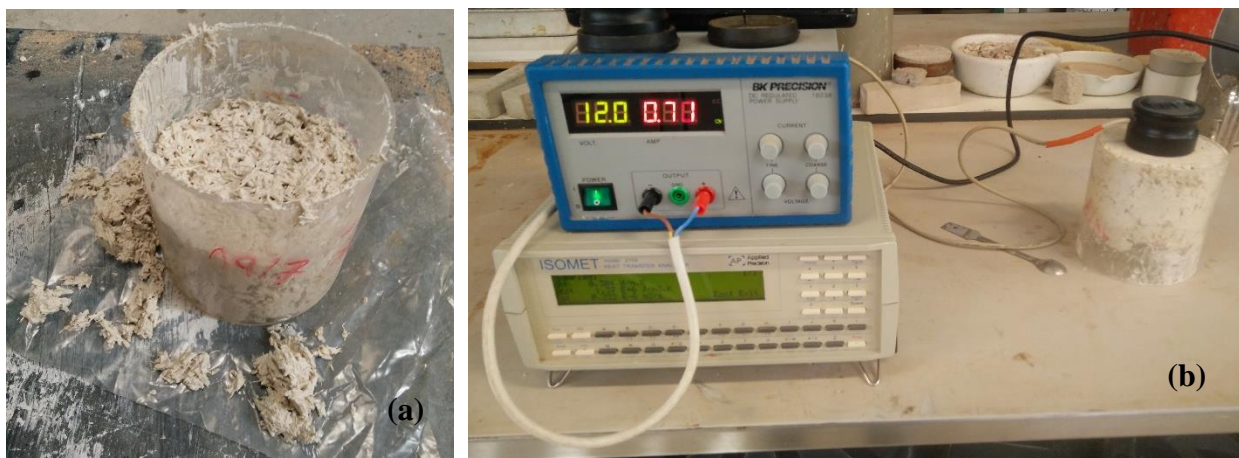
Figure 3.6 – Hemp-lime sample (a) and thermal conductivity determination (b)
