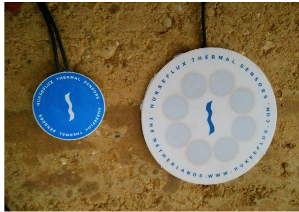
Figure 3.12 - Heat flux plates: HFP01SC (left) and HFP03 (right)
