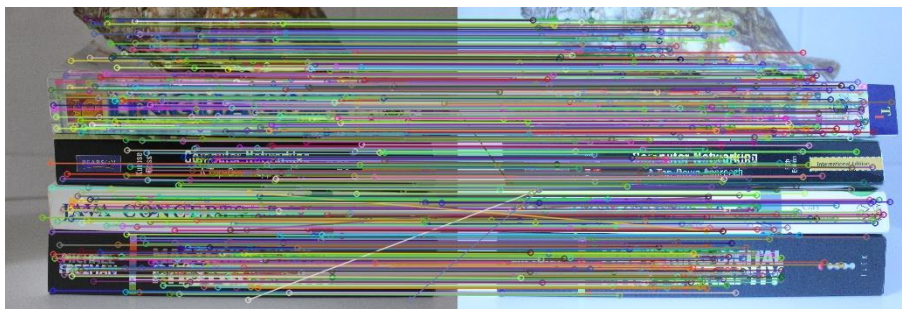
Figure 3.12: Method knnMatch using 1/1.5 as a local threshold.
