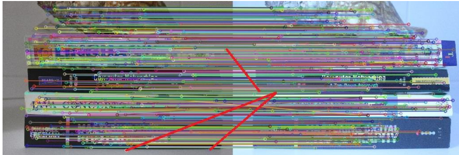
Figure 3.13: FLANN: Three false matches marked in red colour.
