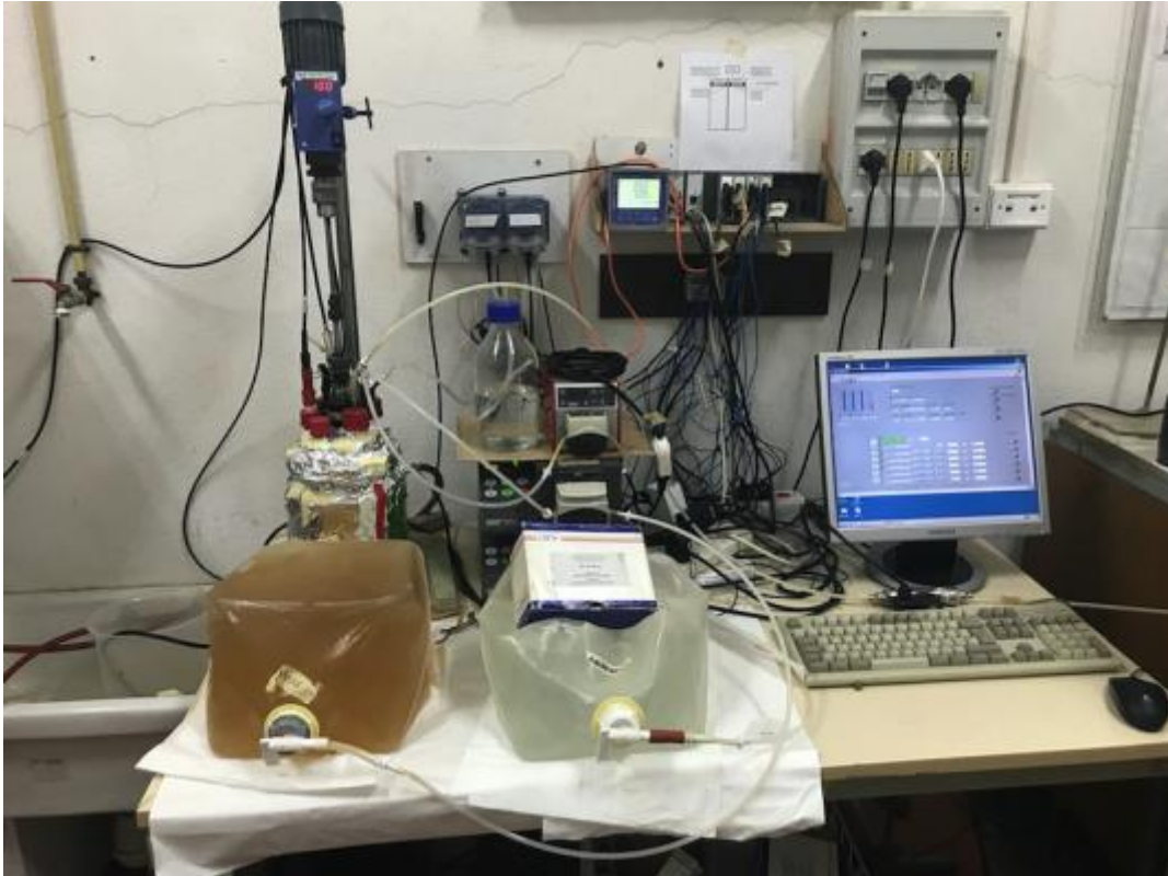
Figure 8 - The Anammox reactor – Experimental set-up
