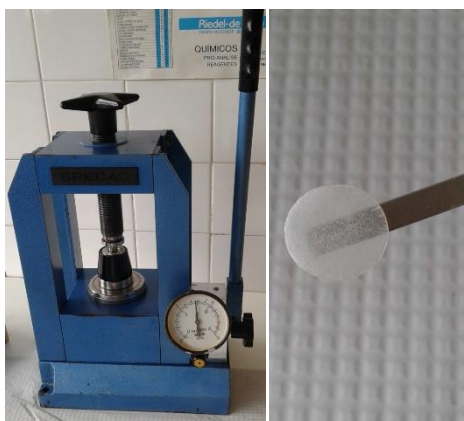
Fig. 2.3. – FTIR tablet preparation using KBr as a solid solvent.
