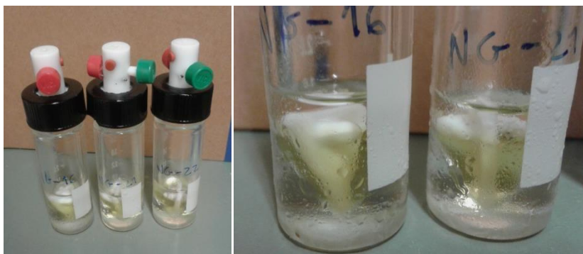
Fig. 3.57. - Reactors with acetonitrile, model oil and standard solution used in the study of the Homogeneous catalysts in ODS.
