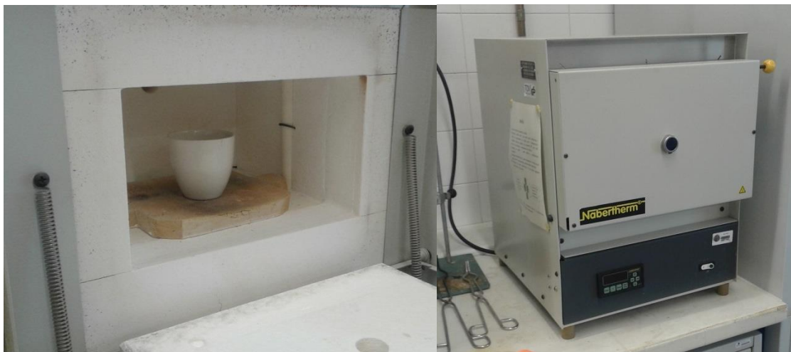
Fig. 2.1. – Calcination of Mesoporous Silica Nanoparticles (MSNPs) at 550 °C for 5 h, using a heating rate of 1 °C/min.
