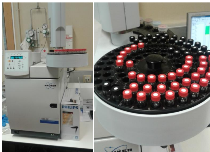
Fig. 3.61. - Gas Chromatograph used to analyze the ODS samples.
