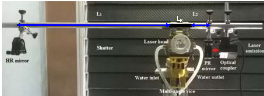
FIG. 7.5 - The solar laser head within the asymmetric resonator.
