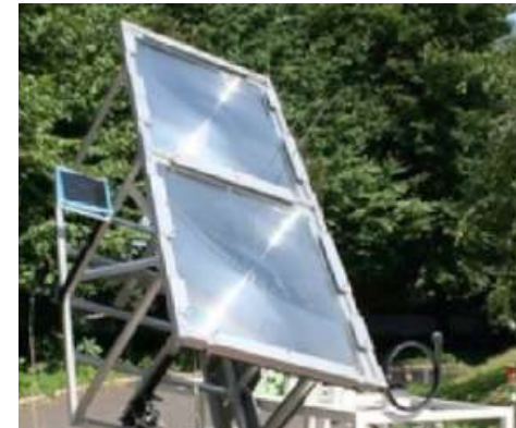
FIG. 2.19 - Test system for laser from natural sunlight (26).
