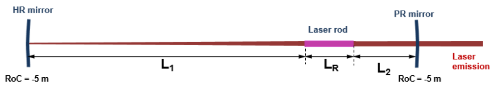
FIG. 2.7 - Schematic diagram of the TEM_{00} -mode beam propagation along the asymmetric laser resonator with large RoC (radius of curvature) end mirrors. L_1 and L_2 represent the separation length of the high reflection (HR) mirror and partial reflection (PR) mirror, respectively, to the end face of the laser rod with length L_R .
