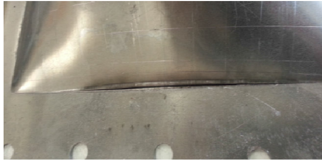
Figure 6. 5 - Mode II tearing at plate experiment 11.
