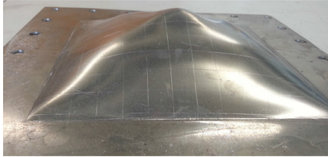
Figure 6.9 - Illustration of the presence of a cap in plate specimens subjected to larger loading and closer stand-off distances.
