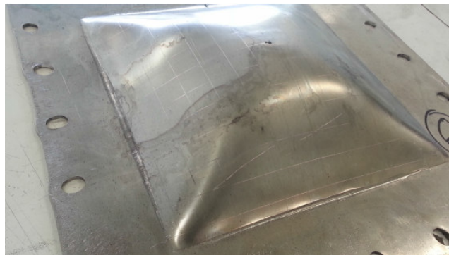
Figure 6. 6 - Thinning and stretching at the plate boundaries in experiment 6
