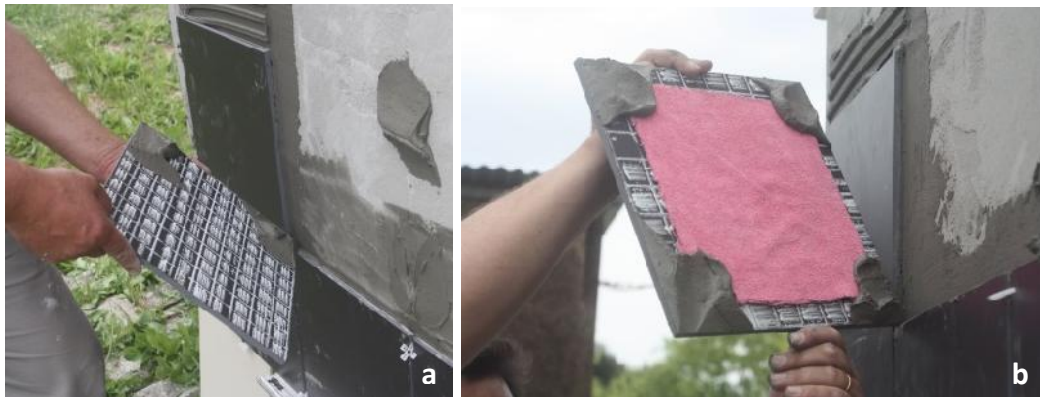
Figure 2 – Simulation of the anomalies of detachment (a) and placement of the water absorptive cloth beneath a tile (b)
