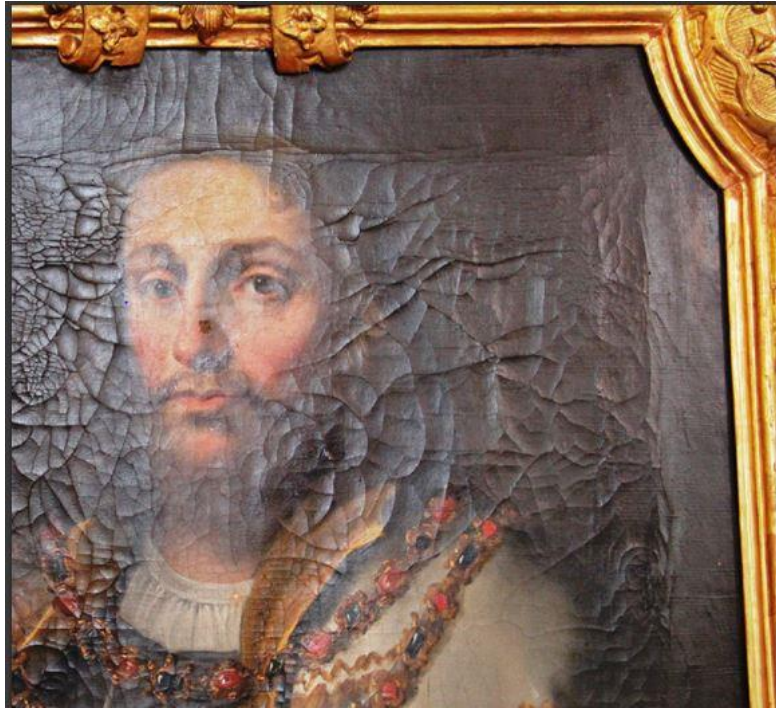
Figure 3.4 - Crack variations related to climate fluctuations. Credit: Stefan Michalski, CCI, adapted from [49]
