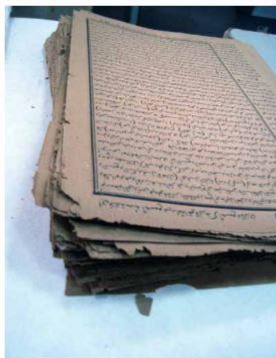
Figure 3.1 - Embrittled low-quality paper, a chemically unstable material that deteriorates notably faster at warm temperatures adapted from [39]
