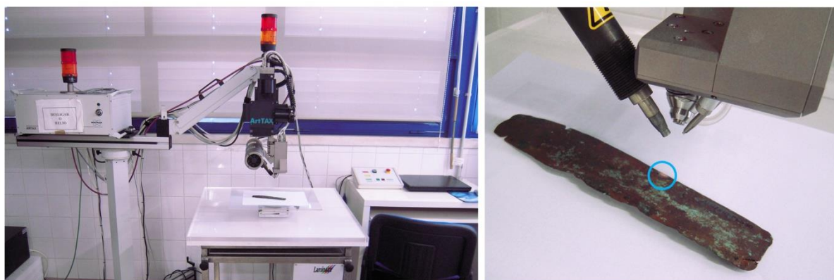
Figure 2.5. Micro-EDXRF spectrometer installed at DCR and example of spot area of the artefact analysed.
