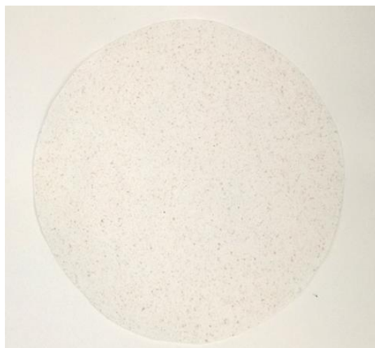
Figure 66 - Paper sheet with DCMC added at a concentration of 18% (w/w). The spots scattered along the sheet correspond to the added DCMC.
