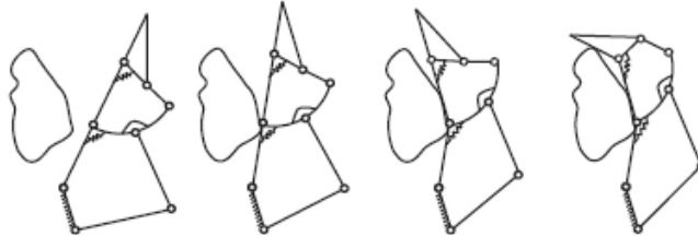
Fig 2.2: Schematic exemplification of the motion from a five-bar mechanism against an object (Taken from [2])
