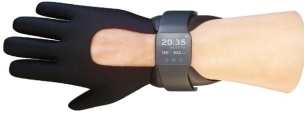
Fig 2.7: Example of an exoskeleton glove with actuators controllers and power systems incorporated in to the glove (Taken from [11])
