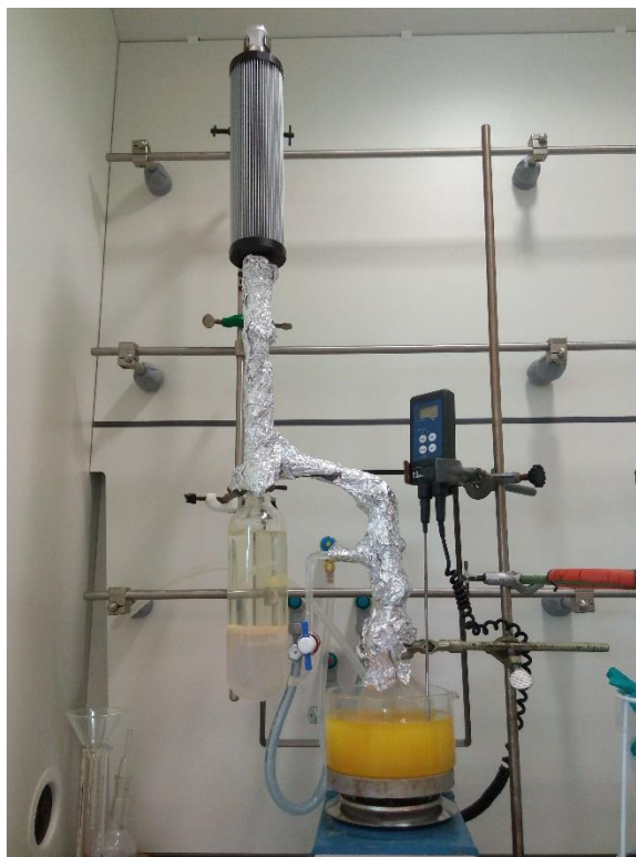
Figure C.1 Preparative scale continuous liquid-liquid extraction using the supernatant from biotransformation and DCM as extracting solvent.
