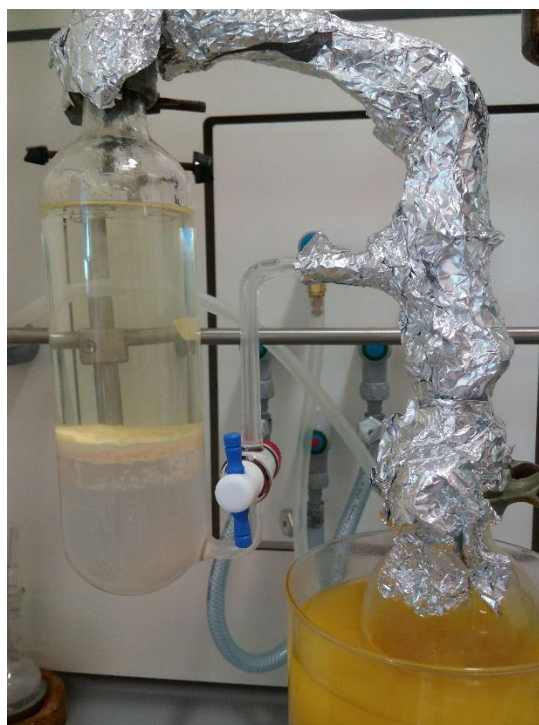
Figure C.2 Zoom-in of the preparative scale extraction. Left: flask with supernatant from the biotransformation on the top and DCM on the bottom. Right: flask with DCM being heated in oil bath.
