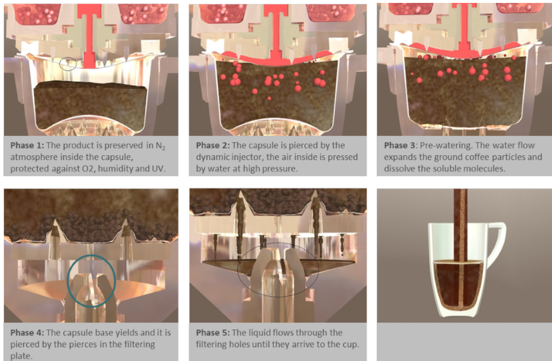
Figure 1.3 – Illustration and description of the different phases of the espresso brewing process of the Monodor capsule system.
