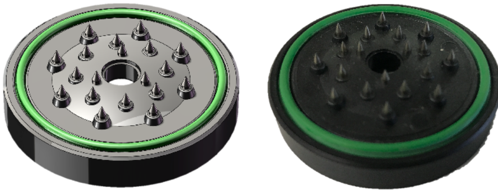
Figure 4.1 – Model of the injection head built in Solidworks (left) and the real life component found inside the device (right).
