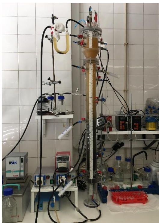
Figure 5.2: Acidogenic fermentation set-up.
