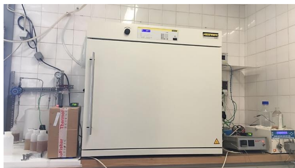
Figure 3.2: SCW apparatus used for BSG hydrolysis.
