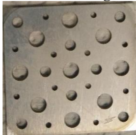
Figure 2.3 Mask used in the aluminium thermal evaporation. Holes with three diameters: 1\text{ mm} , 2\text{ mm} and 3\text{ mm} .
