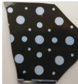
Figure 3.5 - Representative sample with MIS structures having several metal diameters, namely 1 mm, 2 mm and 3 mm.
