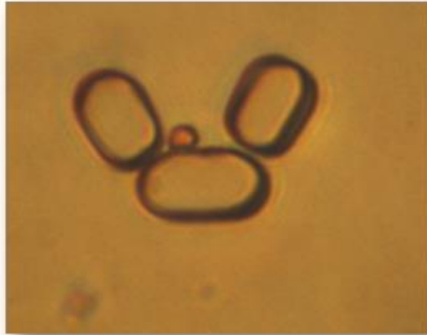
Figure 3.23 – Visualisation of cell trapping. A single-cell was stuck in trap with two opened gaps. The image was acquired with a magnification of 400x in bright field.
