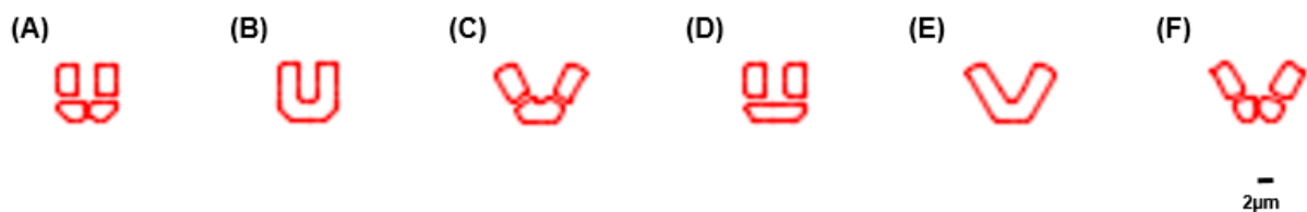
Figure 3.22 – Different structures of designed traps. The traps (A) to (F) were designed and tested on chip to perform the biological assay.
