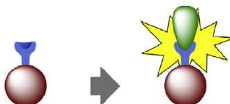
Figure 1.16. Schematics of a standard nanoparticle sensor composed of AuNP (red), recognition molecule (blue), and analyte (green) 12 .
