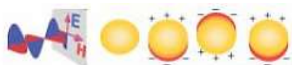
Figure 1.2. Electromagnetic radiation interacting with a nanosphere. Adapted from 5 .
