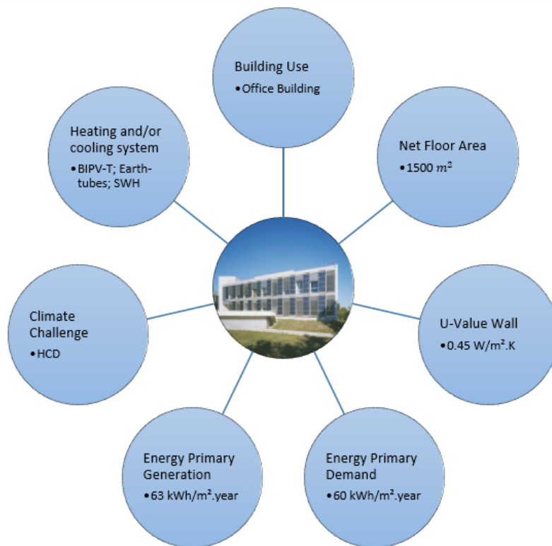
Figure 3.5: Scheme composing Solar XXI main characteristics [26]
