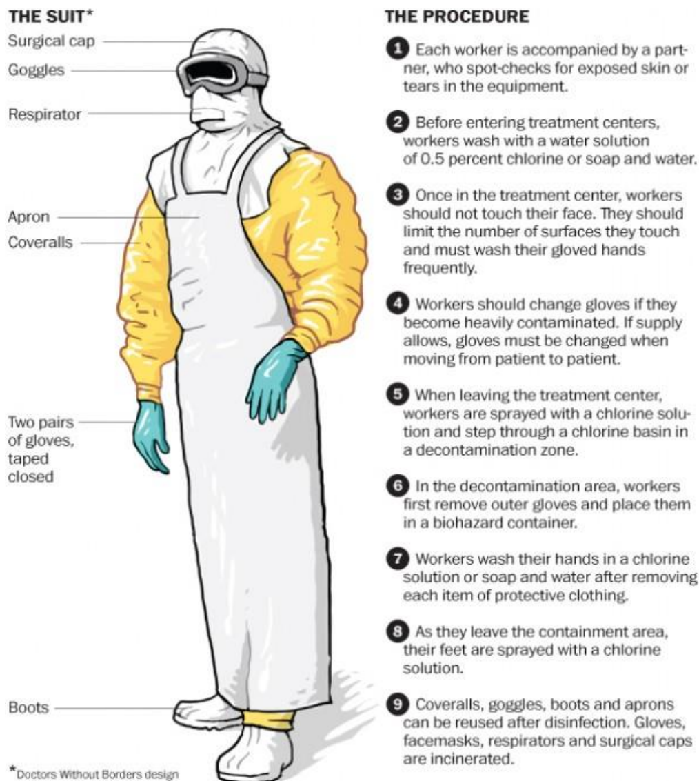
Fig. 2 The materials that constitute the PPE, according to the Médecins sans Frontières (MSF) design, and some rules and instructions regarding the PPE. 6
