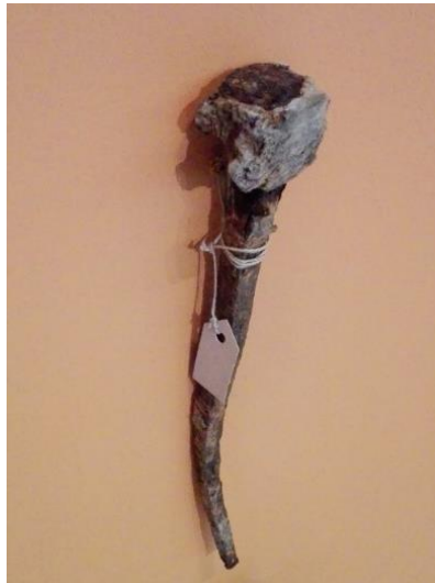
Figure 5.1 - Example of the nail used in the Pombaline buildings exhibited at Museu do Dinheiro – Banco de Portugal
